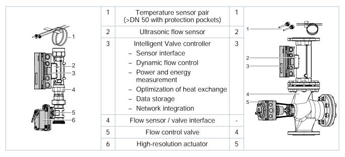
Volume flow is acquired continuously in the ultrasonic flow sensor and provided to the Intelligent Valve controller, where the controller applies it as the actual value for control or limitation by guiding the control valve position until achieving the volume flow actual value for the applicable setpoint.
