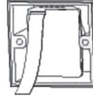
Place Back cover over junction box, insert and tighten mounting screws.
